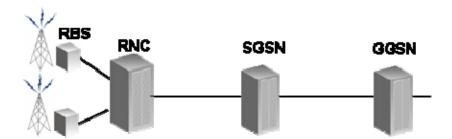
IP packets are sent in packet switch data channels over the radio network. To increase the success rate of fax calls it's important to have a connection with as little as possible latency and jitter since, despite T.38, Fax devices are sensitive to timing. WCDMA is a minimum requirement, but it's recommended to have a HSPA connection since this reduce the latency and jitter. Future radio network improvements, mainly regarding QoS, the fax transmission success rate will further improve.
